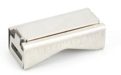
**Universal Channel Clamps** are heavy-duty mounting brackets designed for securing various fixtures, such as signs, enclosures, and equipment, to poles and other vertical structures of different shapes and sizes. These clamps utilize stainless steel banding (sold separately) to attach firmly to the structure, eliminating the need for drilling. The clamp features a robust channel body with slots for the banding and an integrated bolt or threaded stud for attaching the desired fixture.
